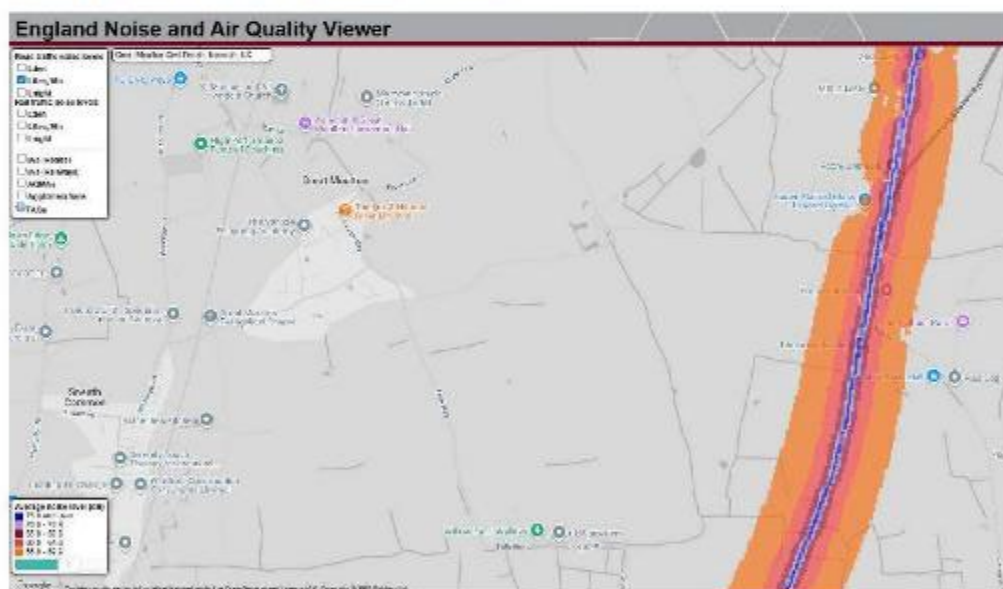
Figure 2 LAeq,16hrs road traffic noise levels (daytime) from Extrium
